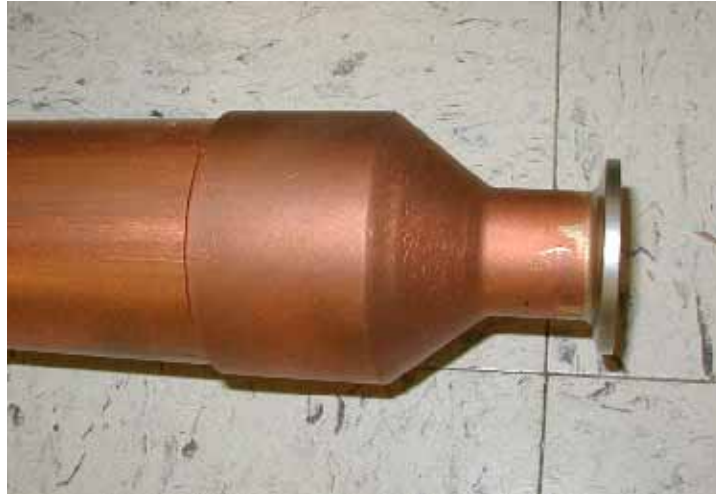
Figure 5-6. Photograph of k-flange to 2” adapter provided by ONI. The adapter is to be soldered to 2” copper tube positioned at a location specified in Figure 5-1 and Figure 2-1.
